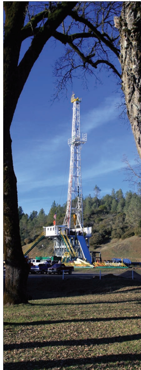
ThermaSource has been working to make its rigs and operations as compact as possible and says it would like to be able to get in a 200-ft-by-300-ft location and still do multiple wells.
