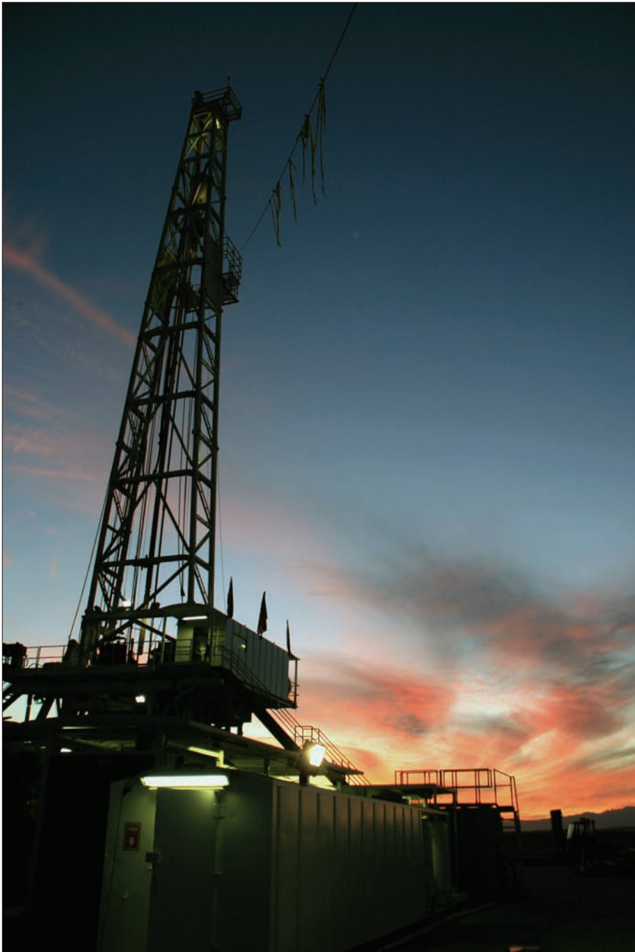
Geothermal drilling rigs are largely similar to oil/gas drilling rigs. They need few, if any, modifications to go from drilling geothermal to drilling for oil or gas.
