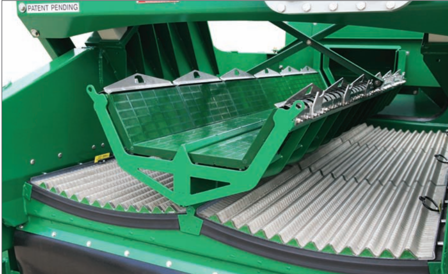
Derrick Equipment's Dual Pool series of shakers can provide 50% more performance over existing shakers in virtually the same footprint, according to the company. The Dual Pool unit uses two screens in reverse crown with the screens in compression rather than tension.
