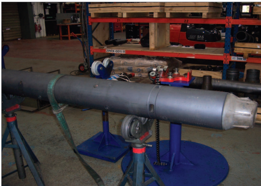
Marathon Oil has been working with partners to adapt radio frequency identification (RFID) technology for use in the oil and gas industry. A tool developed in this effort is the circulating sub, which is activated by passing pre-programmed RFID tags through.
