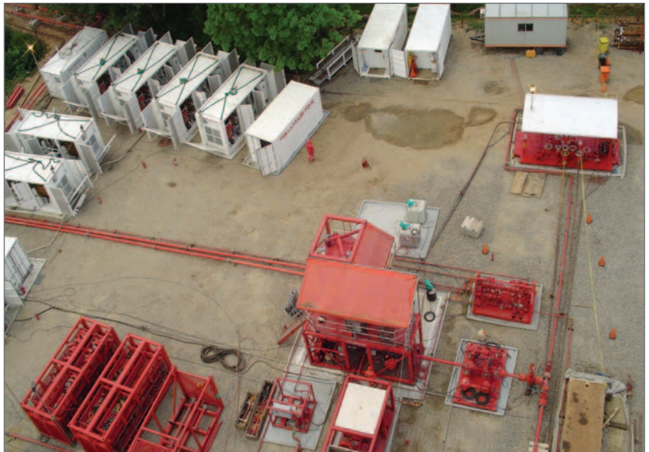
MPD equipment is seen rigged up on location in Southern Mexico, where clean-up times for wells drilled with MPD were reduced from 20 days to an average of 3 days and drilling time was cut in half compared with conventional OB wells.
