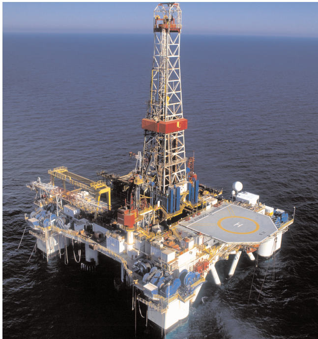
The semisubmersible Atwood Hunter drilled 16 of the 36 wells for development of the West Delta Deep Marine concession offshore Egypt for British Gas in 1998. Other Atwood rigs used in the 4 1/2 year project were Atwood Eagle and Southern Cross. IADC/SPE 87118
