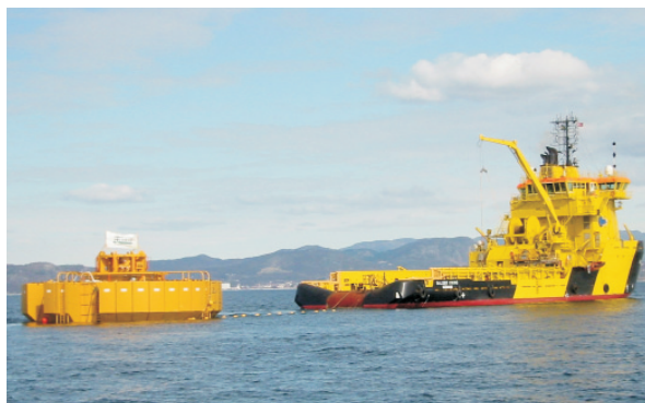
The prototype artificial seabed is towed to a deepwater location off Stavanger for initial field trials.
