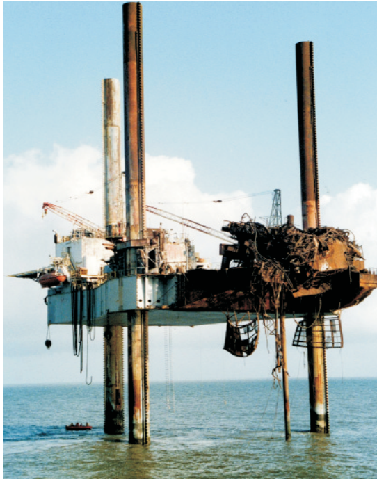
A blowout in the Arabian Sea resulted in a total loss to the drilling package. Capping operations were completed and workers were preparing to plug and abandon the well.
