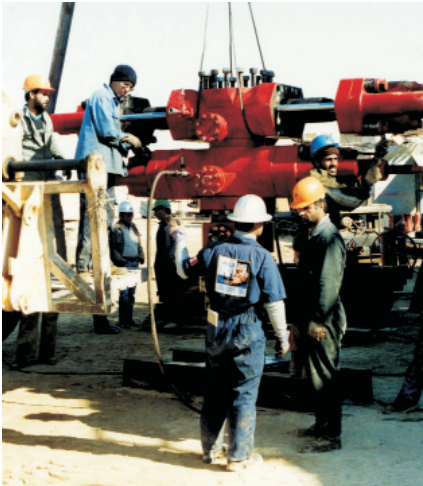
ALERT Disaster Control employees work with a drilling crew to prepare a capping stack for a well control operation in North Africa.
