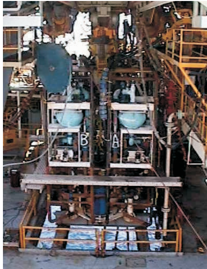
The SubSea MudLift drilling system was brought through the Ocean New Era's moonpool with literally inches to spare.
