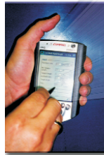
Figure 1: Toolkit user selects tool, inputs data, and receives results. The Driller's Toolkit includes 4 major drilling-engineering categories and 18 subcategories.
