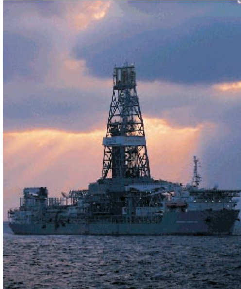
Transocean Sedco Forex drillship Discoverer Enterprise has 20-40% time savings using dual activity concept.
