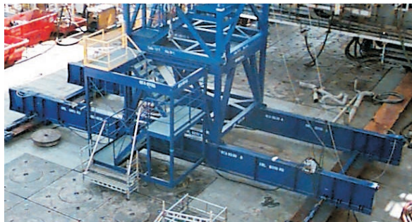
BJ Services' CTD tower has two separate skidding systems. One is for the main structure, shown here, and one for the injector.
