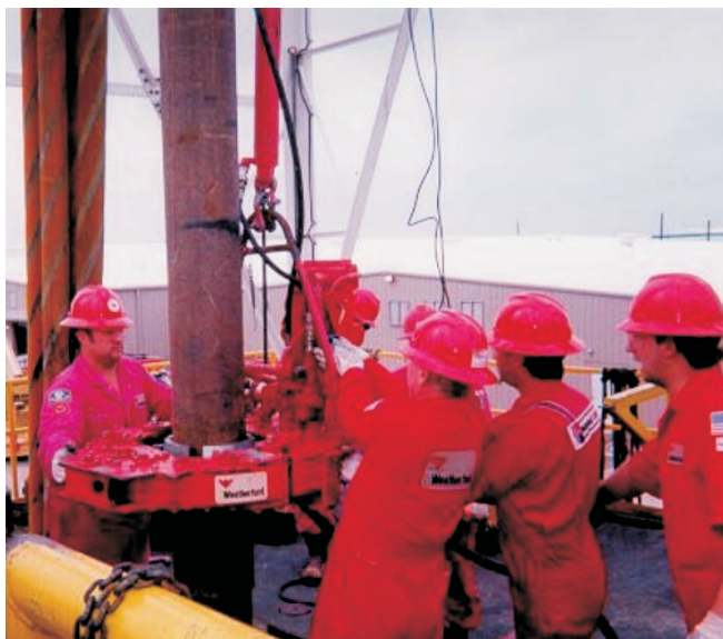
A casing crew receives training on safe and efficient casing running procedures at Weatherford International's Training Center in Houston, Texas.
