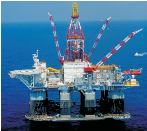
Diamond Offshore's conversion of a North Sea accommodation unit resulted in the deepwater semisubmersible rig Ocean Confidence.
