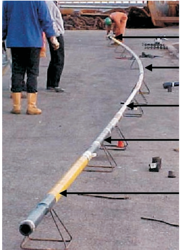
Figure 2: 3½-in. flexible drilling assembly includes, beginning with top arrow, Mach XL motor (BHI), Slimpulse MWD (Anadrill, resistivity tool (TARGET), filter sub (BHI) and thruster (BHI).
