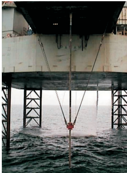
Conductorless drilling of "throwaway wells" used BOP suspended by overhead winches.
