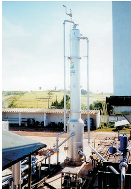
Onshore test in a 1,300-m well was done before taking aerated fluid system offshore
