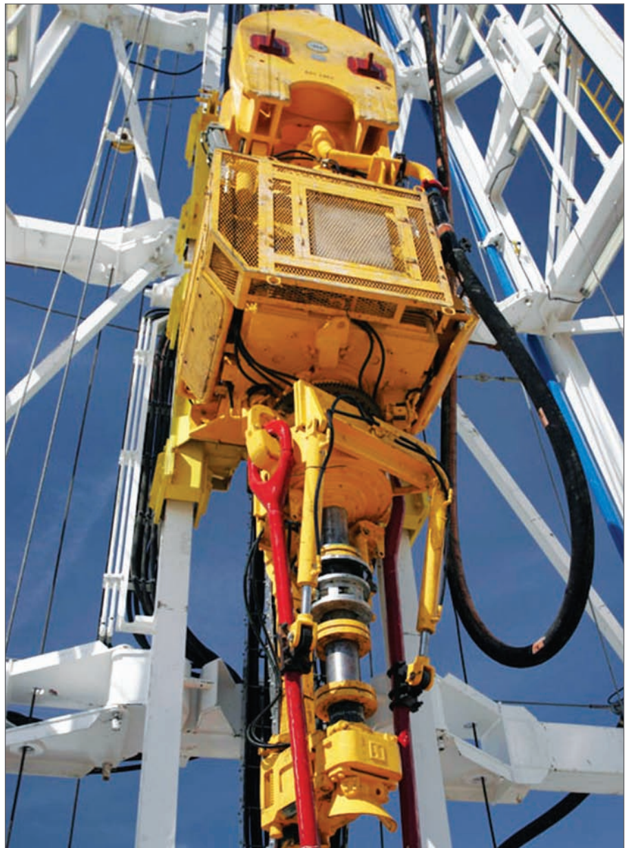
LeTourneau Technologies' DirectDrive top drive system eliminates the gearbox and utilizes an AC motor that delivers up to twice the peak torque as conventional AC motors. The company said it tried to simplify all parts of the system's design.
