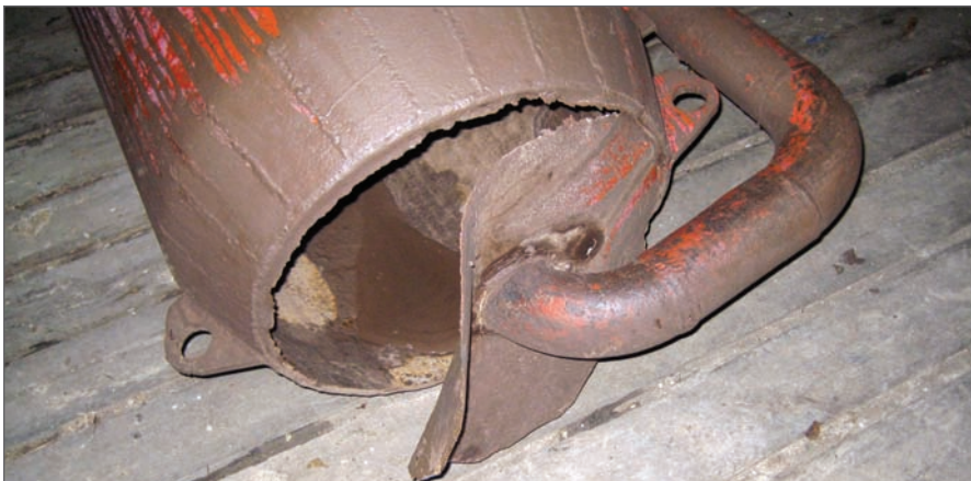
At left, a failed MGS due to excessive pressure.
