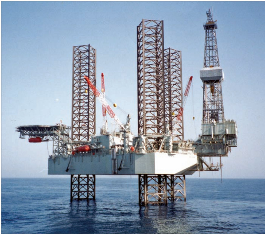
The highly faulted GOT subsurface demands complex 3D directional wells, typically batch drilled, some as deep as 17,000 ft. Above is Transocean's GSF Compact Driller.
