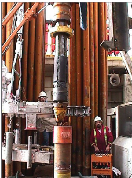
A TESCO casing drive technician assists the driller in stabbing the CDS into the next joint of casing. The casing running operation is completely automated.
