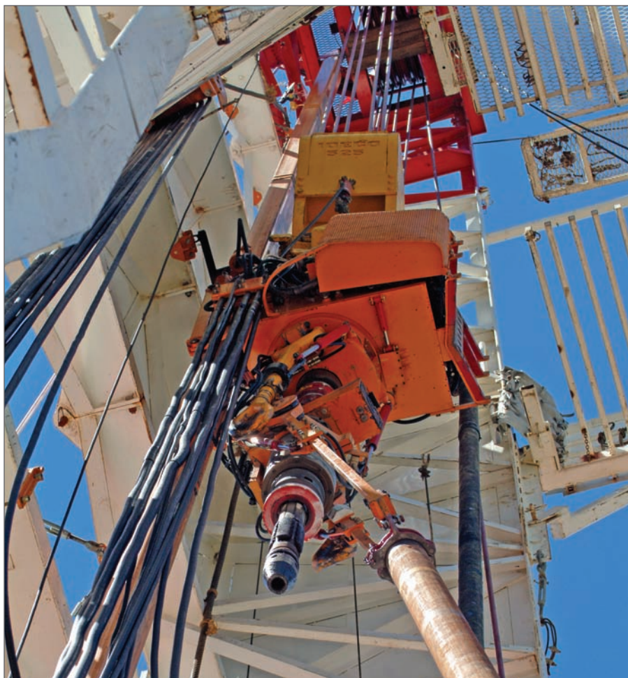
The 12-ft Casing Drive System from TESCO Corp is rated up to 500 ton and makes up directly to the saver sub under any modern top drives.
