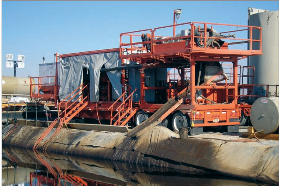
The RECLAIM technology was recently used in a successful field trial in Wyoming that proved its economic value. The package was trailer-mounted and included the RECLAIM unit, a generator and a CD500 centrifuge with stand.
