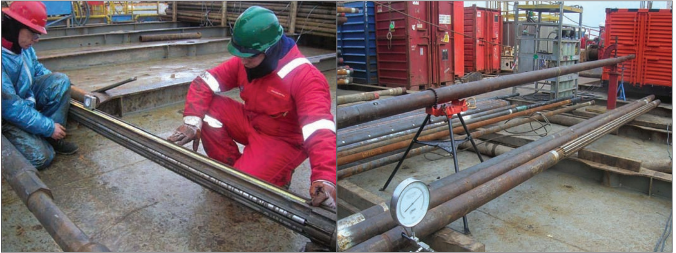
Figure 5: The Armada tubing conveyed sampling system was designed for cased-hole environments.
