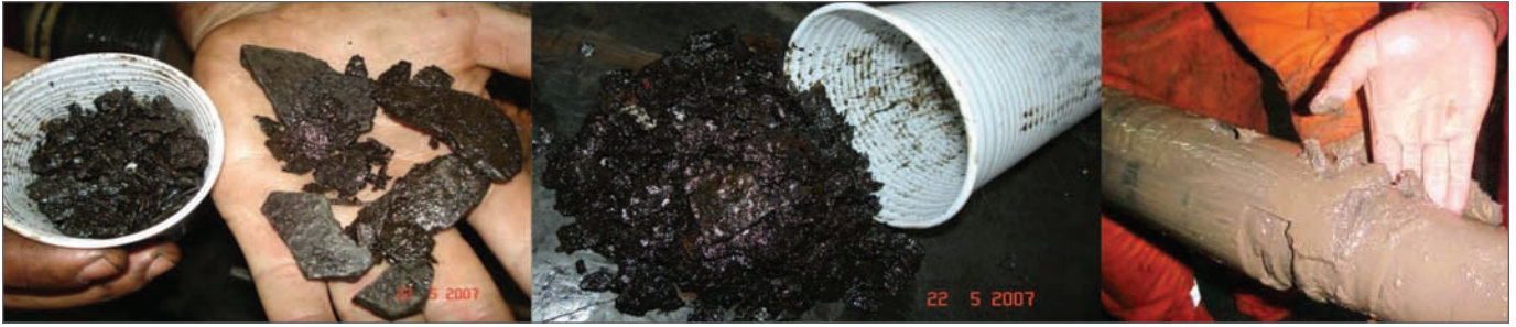
Figure 2: Examples of solids found on the tools used during well testing evaluations.
