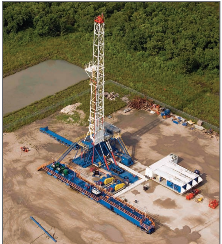
The Fast Moving 1300HP AC VFD rig is one of the most automated, advanced-technology designs from HongHua America, the company said. It is highly mobile and can be moved in 22 loads.
