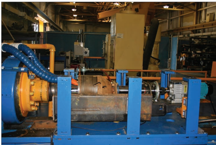
Figure 4: Third-generation hardband test machine with multiple improvements.
