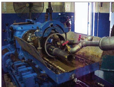
Figure 3: First-generation hardband test machine according to DEA-42.
